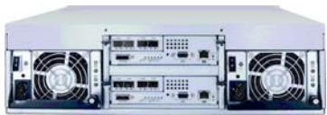
VX-3428R with 8 Fibre Channel 8 Gb ports.
