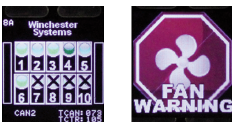
The "X" indicates drives not present and the "fan warning" indicates fan failure.
