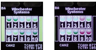
Canister LCD displays drive status including internal temperatures. Red indicators signify failed drives.
