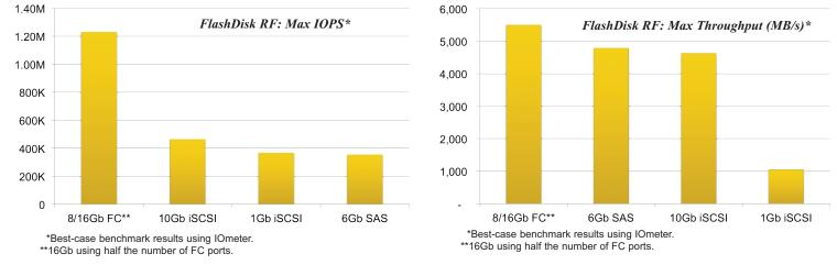
Both FlashDisk RF and RV come in 2U and 3U rack-mount sizes, and support 2.5" and 3.5" SAS hard disk drives and SSDs. FlashDisk RV systems are also available in a 1U size. Host interconnect options include 8 or 16 Gbps Fibre Channel, 1 or 10 Gbps iSCSI, and simultaneous Fibre Channel and iSCSI.
