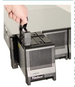
FX-4U60 offers easy access to top-loading drives with three separate drawers for convenience and safety.
